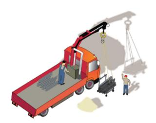
Initially use pallets, stilages and frame containers when you are going to move the elements of the scaffolding from a storage site to a vehicle and from the vehicle to the site where the scaffolding is to stand.
